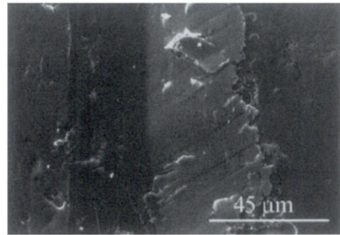
Fig. 21 Surface fracture behavior of n WC-15%Co during scratch test
